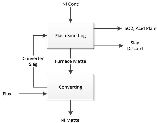
Figure 1. Nickel matte production by flash smelting at Vale Sudbury
