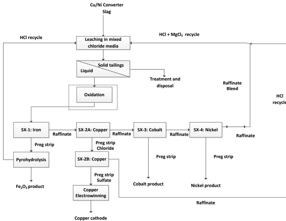
Figure 6. PRO flowsheet for treatment of Cu/Ni converter slag
