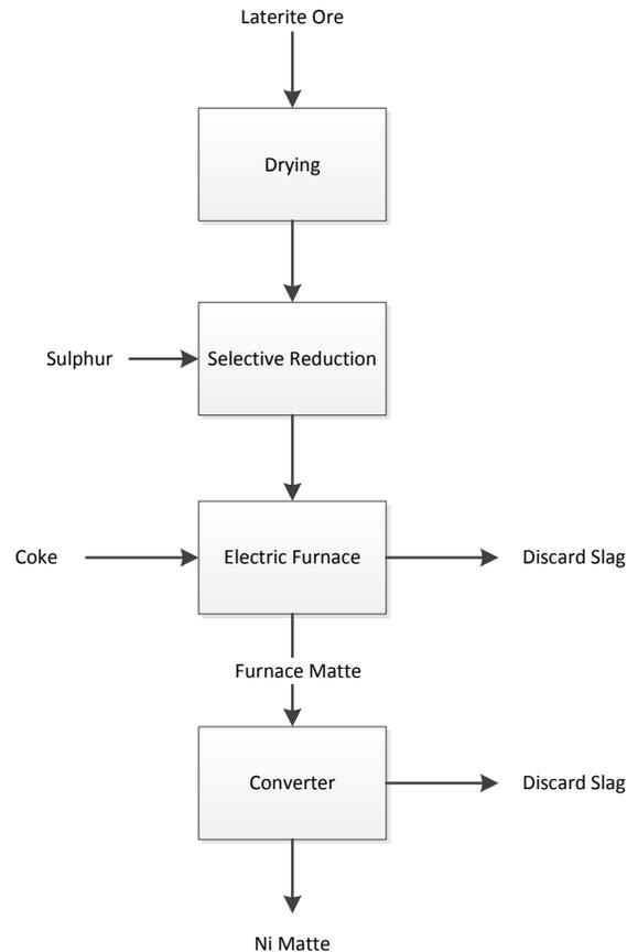
Figure 7. Vale laterite smelting process to make nickel matte
