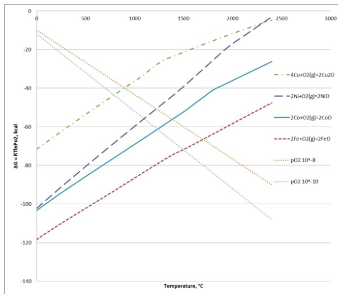
Figure 4. Free energy of formation of Cu, Ni Co and Fe oxides
