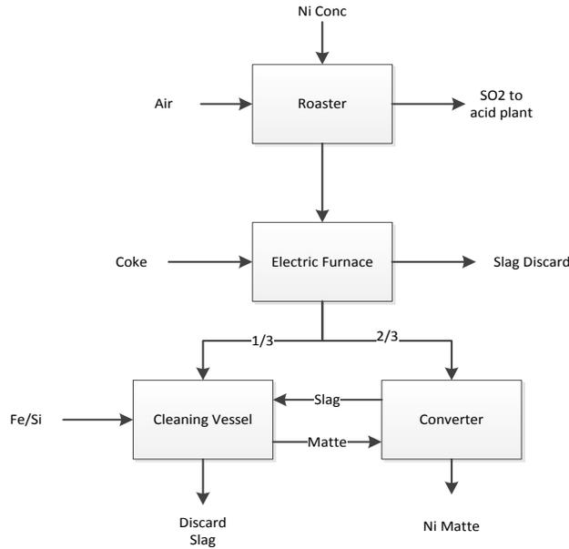
Figure 2. Nickel matte production by roast-reduction by Glencore at Sudbury
